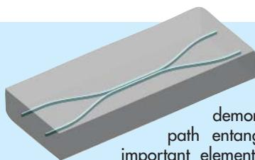
splitters, interferometers, and even a controlled-NOT gate, but combined those devices into photonic circuits. Among their demonstrated results is a high-fidelity, path entangled state of two photons, an important element for quantum computation. The silica-on-silicon photonic circuits may also be applied to quantum metrology and communication technologies. (A. Politi et al., *Science* **320**, 646, 2008.) —JNAM
