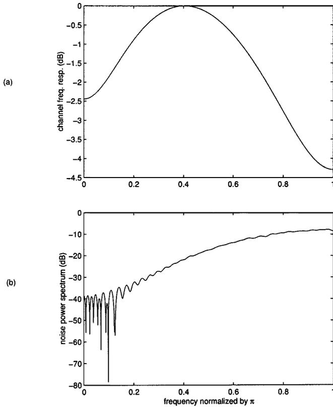
Fig. 5. (a) Frequency response of the channel  $|C(e^{j\omega})|$ . (b) Power spectrum of the channel noise  $\nu(n)$ .
