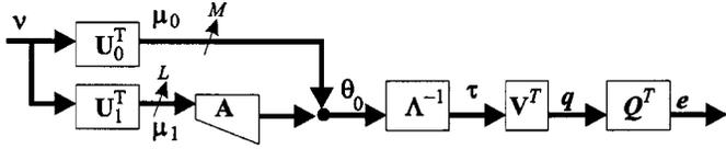
Fig. 3. Receiver in the form of  $\mathbf{S} = \mathbf{Q}^T \mathbf{V}^T \mathbf{\Lambda}^{-1} [\mathbf{I} \ \mathbf{A}] \mathbf{U}^T$  for the derivation of an optimal  $\mathbf{A}$ .
