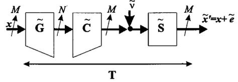
Fig. 4. Matrix representation of DMT systems with a general prefix.
