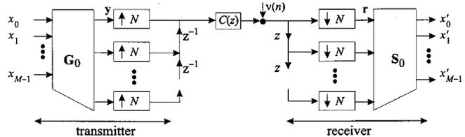
Fig. 1.  $M$ -band block-based DMT transceiver over channel  $C(z)$  with noise  $\nu(n)$ .
