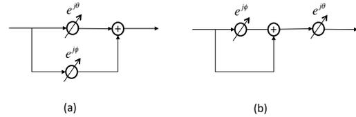
Fig. 2. Phase shifter implementation, (a) Structure I, and (b) Structure II.
