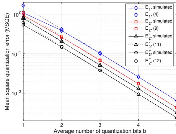
Fig. 3. Mean square quantization error as a function of  $b$ , the average number of quantization bits.
