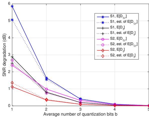
Fig. 5. Average SNR degradation as a function of  $b$  for a beamforming system with  $N_t = N_r = 16$ .
