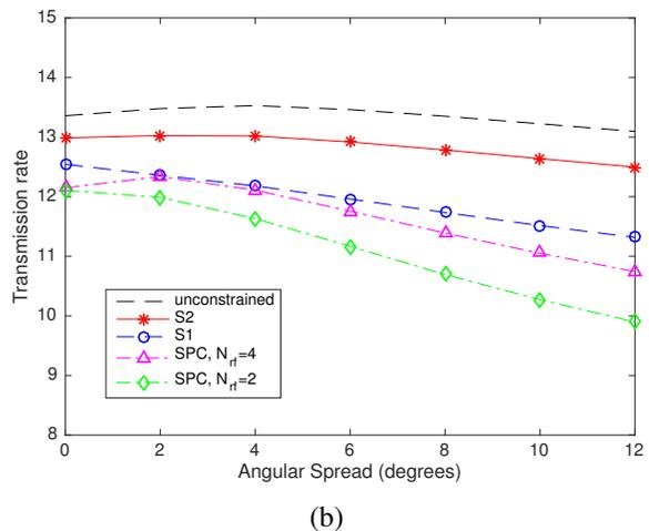
Fig. 6. Hybrid precoding system with  $N_t = N_r = 64$  and  $N_s = 2$ ; (a) transmission rate vs. SNR, and (b) transmission rate vs. angular spread.
