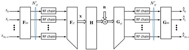
Fig. 1. A MIMO communication system with hybrid precoding.
