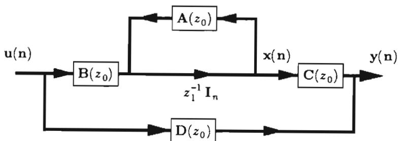
Figure 8.2. The schematic of the first-level description for  $E(z)$ .
