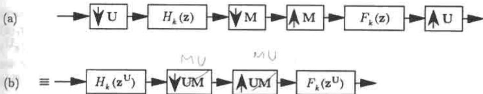
Figure 3.6. Derivation of the  $k$ th subband of the new system  $\mathcal{FB}_{UM}$ .
