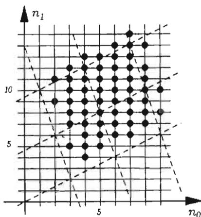
Figure 6.10. Example 6.1. Two-copy cosine modulated filter bank. The impulse response support of the prototype. Each solid dot represents a possibly non-zero coefficient of the prototype. (Intersection points of the dashed lines are on the lattice of  $\mathbf{N}$ . Solid lines represent integers.)
