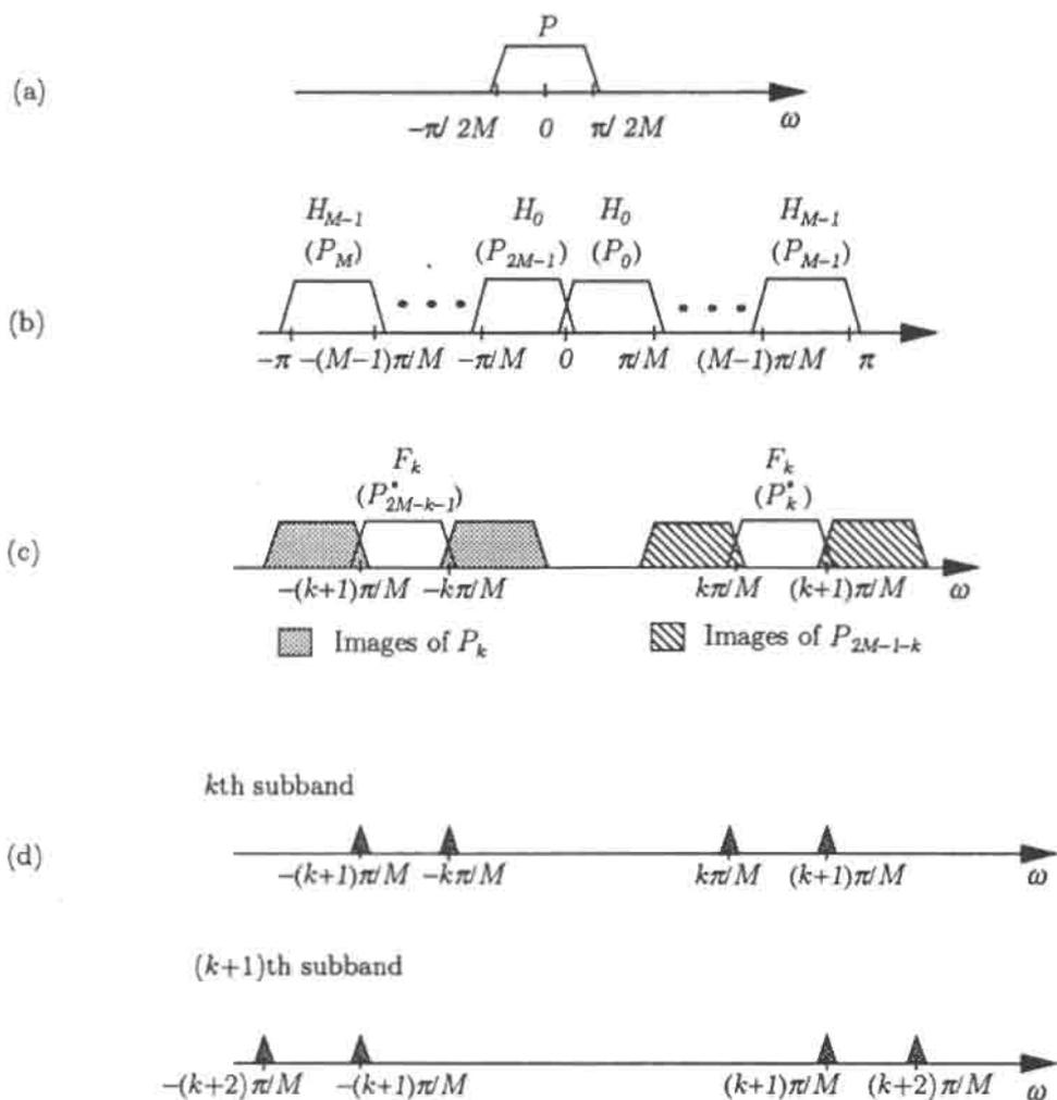
Figure 5.1. One-dimensional cosine modulated filter bank. (a) The support of the prototype filter  $P(\omega)$ . (b) The support of the analysis filters  $H_k(\omega)$ . Each analysis filter has two parts,  $P_k(\omega)$  and  $P_{2M-k-1}(\omega)$ . (c) Images of the analysis filter  $H_k(\omega)$  that are adjacent to the synthesis filter  $F_k(\omega)$ . (d) The major aliasing in the  $k$ th subband and the  $(k+1)$ th subband.
