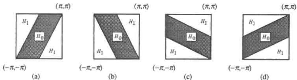
Figure 1.7. Four possible parallelogram supports of the two-channel filter bank.
