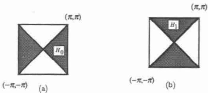
Figure 1.6. The filter bank with fan filters. (a) The support of  $H_0(\mathbf{w})$ . (b) The support of  $H_1(\mathbf{w})$ .
