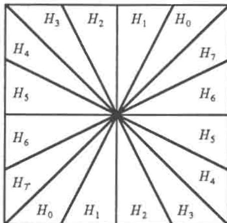
Figure 1.9. Supports of the analysis filters in the directional filter bank.
