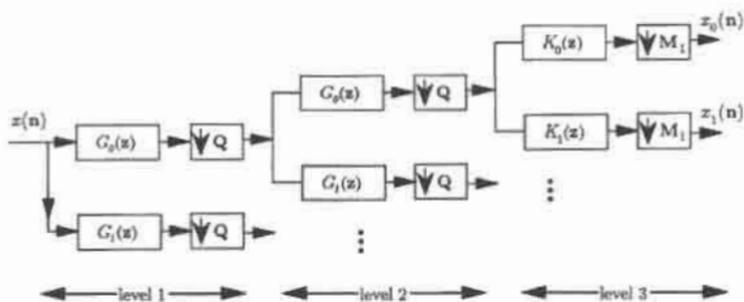
Figure 4.2. Tree-structured filter bank for the derivation of directional filter banks. In the first and second levels, each subband is split into two. Only the first two subbands of the overall system are shown in the figure.
