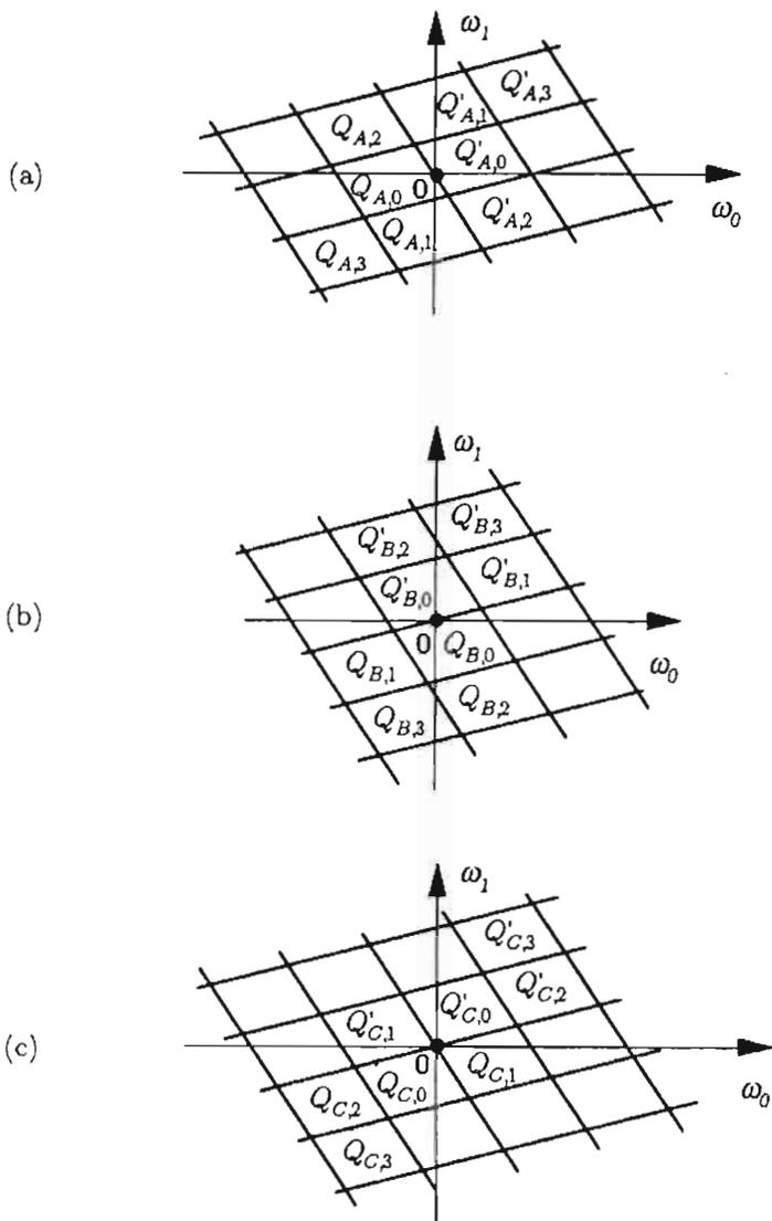
Figure 7.2. Shifted versions of the filters in the DFT filter bank.
