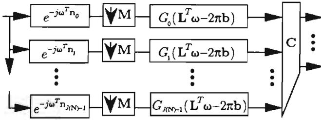
Figure 6.8. Efficient implementation of the analysis bank of the two-copy cosine modulated filter bank. The matrix  $\mathbf{C}$  is of dimension  $|\det \mathbf{M}|$  by  $2|\det \mathbf{M}|$ .
