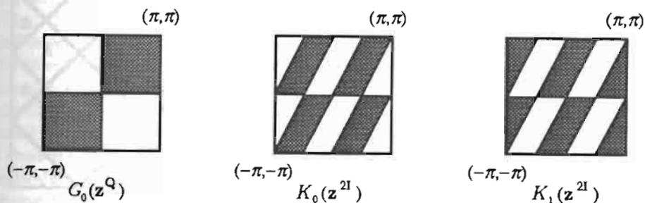
Figure 4.5. The supports of  $G_0(z^Q)$ ,  $K_0(z^{2I_2})$  and  $K_1(z^{2I_2})$ .
