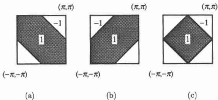
Figure 2.4. The ideal responses of (a)  $(z_0 z_1)^{-1/2} \alpha(z_0 z_1)$ , (b)  $(z_0 z_1^{-1})^{-1/2} \alpha(z_0 z_1^{-1})$ , and (c)  $z_0^{-1} \beta(\mathbf{x}^Q)$  for the diamond filter bank.
