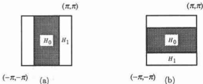
Figure 1.3. Two types of support configurations for separable two-channel filter banks.
