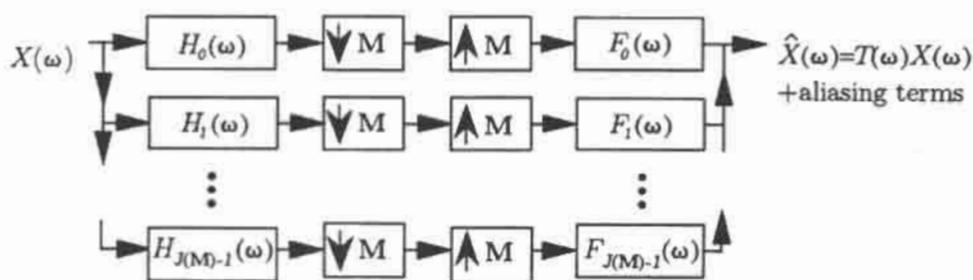
Figure 1.1.  $J(M)$ -channel maximally decimated filter bank, where  $J(M) = |\det \mathbf{M}|$ .
