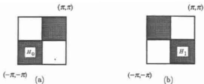
Figure 1.5. The support configuration of the quadrant filter bank. (a) The support of  $H_0(\mathbf{w})$ . (b) The support of  $H_1(\mathbf{w})$ .
