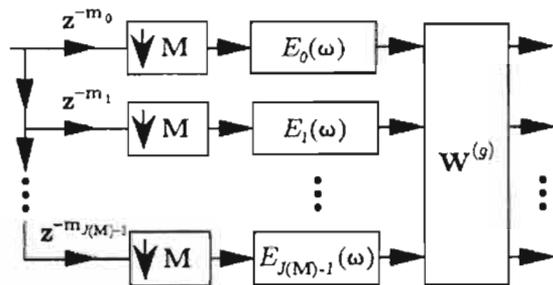
Figure 3.2. The implementation of the MD DFT filter bank, where  $\mathbf{W}^{(g)}$  is the generalized DFT matrix.
