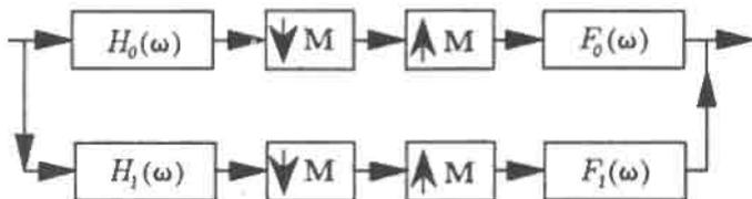
Figure 2.1. Two-dimensional two-channel filter bank, where  $\mathbf{M}$  is a 2 by 2 integer matrix with  $|\det \mathbf{M}|=2$ .
