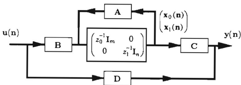
Figure 8.3. The schematic of the Roesser state space description for  $E(z)$ .
