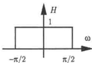
Figure 2.2. The desired response of  $H(\omega)$ .
