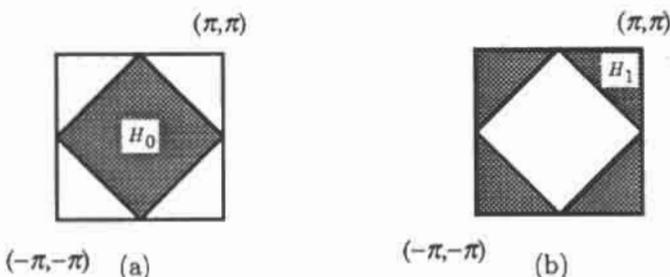
Figure 1.4. The support configuration of the diamond filter bank. (a) The lowpass analysis and synthesis filters. (b) The highpass analysis and synthesis filters.
