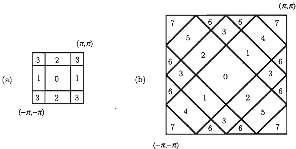
Figure 4.7. Example 4.3. Tree structured filter bank. (a) The first level of the tree: the four-channel separable filter bank. The supports of the four separable analysis filters (with the support of the  $k$ th filter denoted by  $k$ ). (b) The supports of the eight analysis filters in the overall system. The support of  $H_k(z)$  is denoted by  $k$ .
