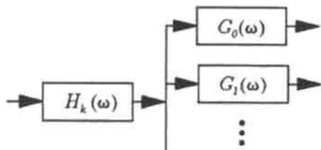
Figure 1.8. Tree structured analysis filter bank. Splitting of the  $k$ th subband.
