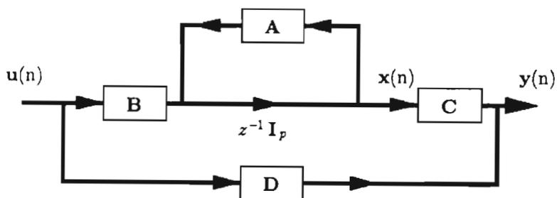
Figure 8.1. The schematic of the state space description for  $E(z)$ .
