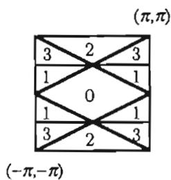
Figure 4.6. Example 4.2. Tree structured filter bank. The supports of the analysis filters. In the figure the support of  $H_k(z)$  is denoted by  $k$ .
