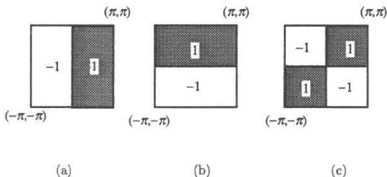
Figure 2.5. The ideal responses of (a)  $jz_0\alpha(-z_0^2)$ , (b)  $jz_1\alpha(-z_1^2)$ , and (c)  $z_0^{-1}\beta(\mathbf{z}^{\mathbf{D}})$  for the quadrant filter bank.
