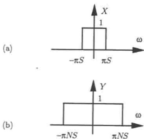
Figure 3.3. Relation of the input support and the output support for an  $N$ -fold decimator. The output  $Y(\omega)$  is a stretched version of the input  $X(\omega)$ .
