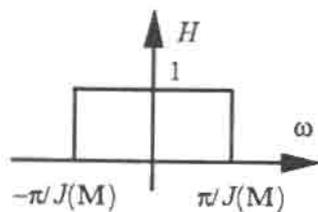
Figure 3.4. The desired response of the 1D filter  $H(\omega)$ .
