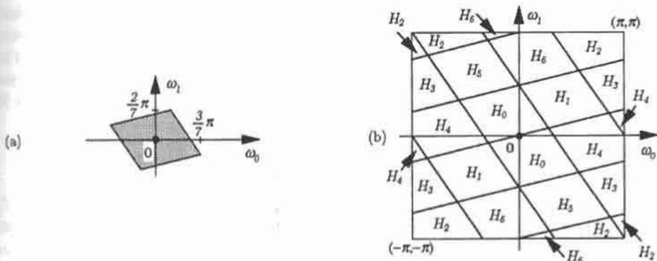
Figure 6.9. Example 6.1. Two-copy cosine modulated filter bank. (a) Spectral support of the prototype  $P(w)$ ,  $SPD(\pi N^{-T})$ , and (b) supports of the analysis filters.
