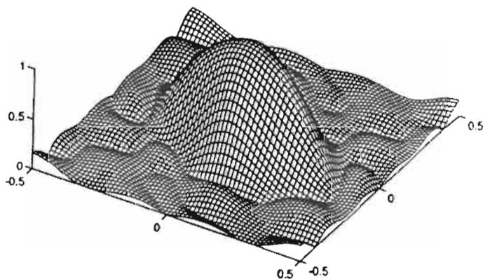
Figure 6.11. Example 6.1. Two-copy cosine modulated filter bank. The magnitude response of the prototype with frequency normalized by  $2\pi$ .
