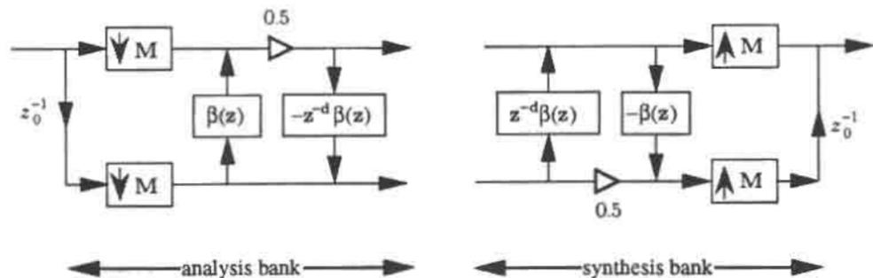
Figure 2.6. The implementation of the diamond filter bank or the quadrant filter bank that is designed through the Nyquist(M) approach.
