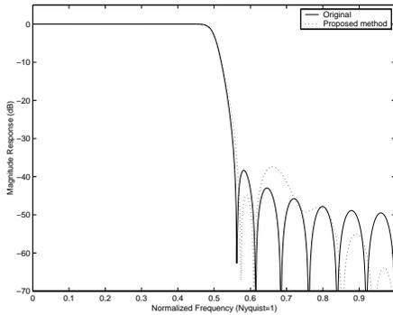
Figure 5: IIR filter quantized by our proposed method using CSD code.
