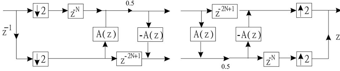
Figure 2: The ladder structure for two-channel filter bank.
