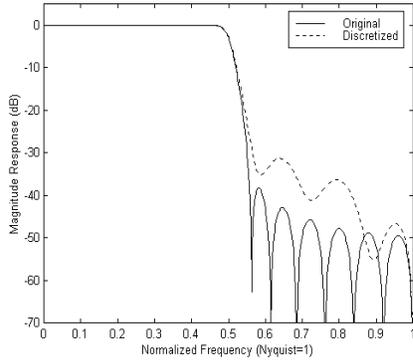
Figure 4: IIR filter quantized directly using CSD code.
