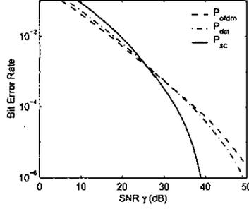
Figure 5: Example 2. The performance of  $\mathcal{P}_{ofdm}$ ,  $\mathcal{P}_{dct}$  and  $\mathcal{P}_{sc}$  over a 4-tap multipath fading channel.
