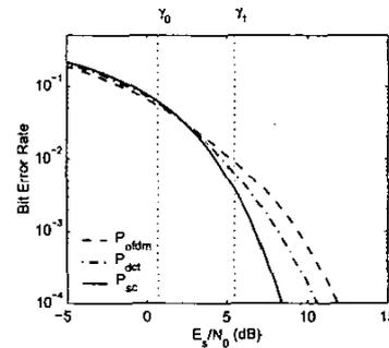
Figure 4: Example 1. Performance comparison of  $\mathcal{P}_{ofdm}$ ,  $\mathcal{P}_{dct}$  and  $\mathcal{P}_{sc}$  systems for the channel  $P(z)$ .
