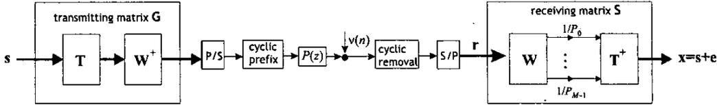
Figure 2: The OFDM system with a precoder  $T$ .
