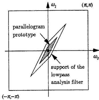
Fig. 7. Simplistic four parallelogram filter bank. The parallelogram prototype  $SPD(\pi N^{-T})$  and the support of the lowpass analysis filter  $SPD(\pi M^{-T})$ .
