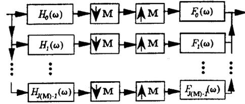
Fig. 1.  $J(M)$ -channel maximally decimated filter bank, where  $J(M)=|\det(M)|$ .
