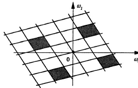
Fig. 4. Typical support of an analysis filter in a four-parallelogram filter bank.
