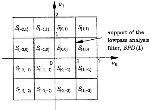
Fig. 8. The support of the lowpass analysis filter (with the frequency plane normalized by  $2\pi N^{-T}$ ).
