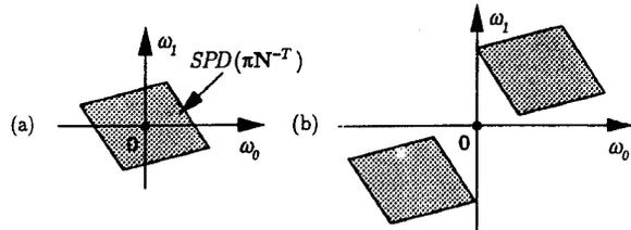
Fig. 2. Two-parallelogram filter bank. (a) Parallelogram prototype and (b) typical support of an analysis filter.
