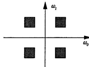
Fig. 5. Separable filter bank. Typical support of an analysis filter.
