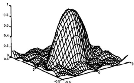
Fig. 6. Example 4.1. Two-dimensional linear phase cosine modulated filter bank. The magnitude response of the prototype with frequency normalized by  $2\pi$ .
