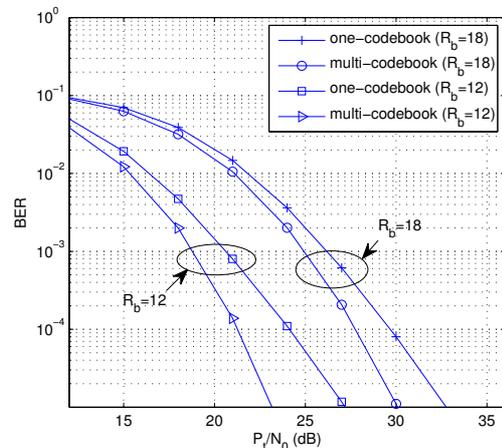
Fig. 2. Example 1. Multiple v.s. one precoder codebooks.
