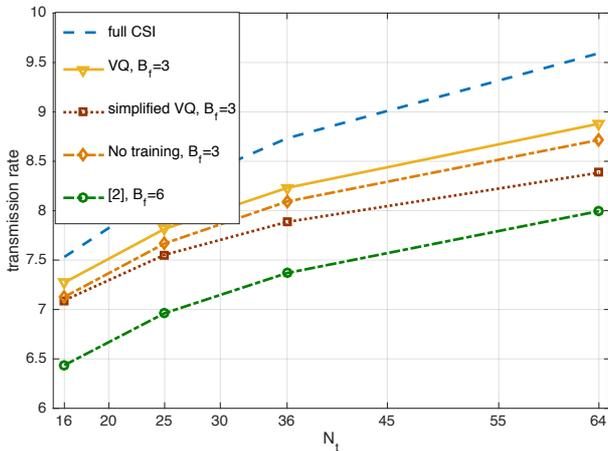
Figure 2: Transmission rate v.s.  $N_t$  (the number of transmit antennas).
